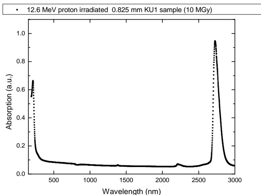
Figure 1. Absorption spectrum of KU-1 sample 12.6 MeV proton irradiated at 30 °C to 10 MGy
