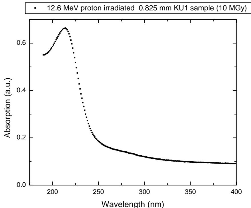
Figure 2. Absorption spectrum of KU-1 sample 12.6 MeV proton irradiated at 30 °C to 10 MGy (magnified region of interest)
