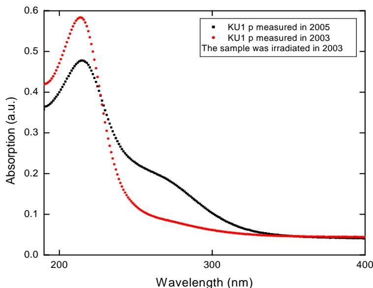
*Figure 5 KU-1 absorption spectra measured in November 2003, respectively in June 2005 on the same sample 12.6 MeV p irradiated in 2003 at 30 °C to 8 MGy*
